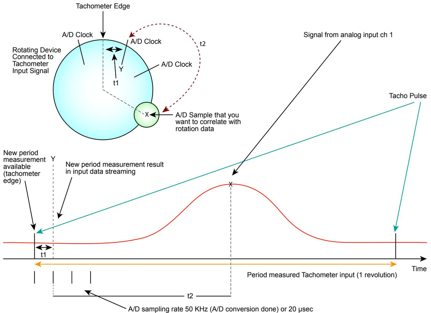
**Figure 7.** By connecting a rotating device to the tachometer input of the DT8837, you can measure the frequency or period of the rotating device. The DT8837 also provides the ability to accurately measure the time between the tachometer edge and the next A/D sample or between the A/D sample and the next tachometer edge, so that you can precisely correlate A/D data with rotation data.
