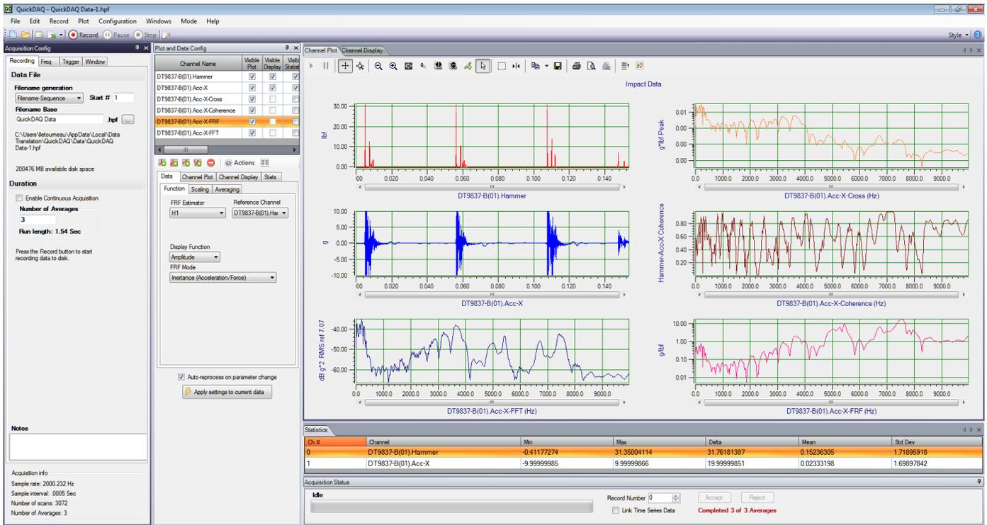
Figure 13. QuickDAQ with Advanced FFT Analysis Option.
