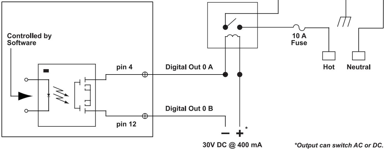
**Figure 8.** The 4 isolated digital outputs offer high drive capability. They are solid state relays that are capable of switching up to  $\pm 30V @ 400mA$ . Either AC or DC can be switched. The internal solid state relays are poly fused to prevent any damage and they restore as soon as a short is removed
