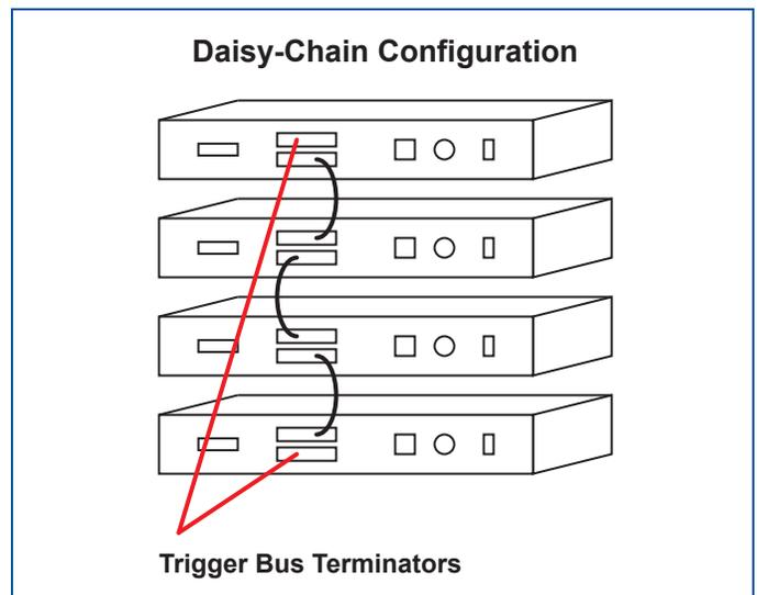
**Figure 9.** Multiple DT8837 instrument modules in daisy-chain configuration
