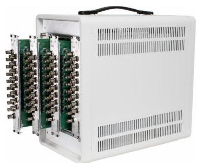
Figure 2. VIBbox-64 packages four DT9857E modules in a rugged enclosure for field use. The user can take advantage of the full expandability of this module series in a self-contained enclosure. The use of a USB hub internal to the system allows easy connection to the host computer through one simple USB cable. An external power supply is included.
