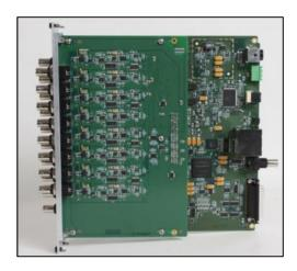
Figure 3. The DT9857E provides sixteen IEPE analog inputs, 2 analog outputs, 16 DIO, 1 C/T, 1 Tachometer, and 2 Measure Counters on each board set. VIBbox-64 packages four of these to bring the channel count to: 64 IEPE analog inputs, 8 analog outputs, 64 DIO, 4 C/T, 4 Tachometers, and 8 Measure Counters. For more information on the DT9857E module, visit our web site: <u>http://www.datatranslation.com/products/</u> <u>dataacquisition/usb/DT9857E/</u>
