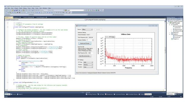
Figure 6. The Signal Processing Component Library for .NET is a comprehensive library of object-oriented classes ideal for developing signal processing applications. Each class contains properties and methods that can be used to perform single-channel and two-channel FFT operations, and to calculate signal metrics on time domain data. This library is included free with VIBbox.
